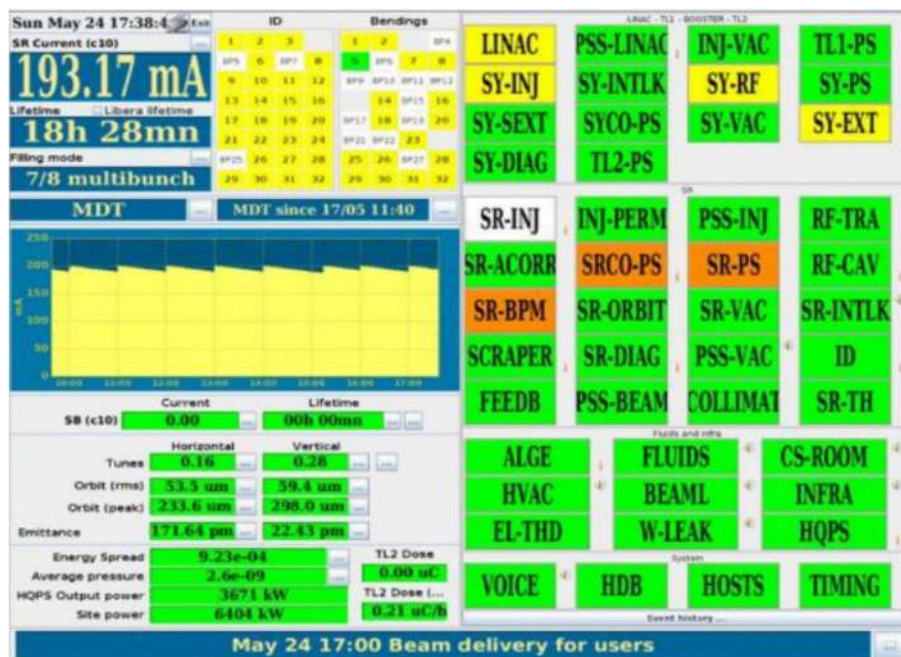
Fig. 15 Commissioning status of ESRF-EBS in 2020
