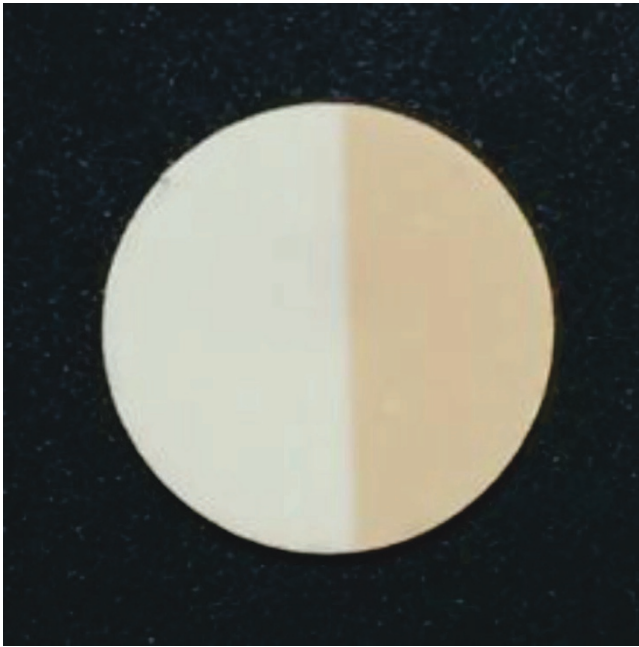
Figure 3 UV-irradiation-induced coloration of the \text{MgGeO}_3:\text{Yb}^{3+} phosphor. Digital picture of an \text{MgGeO}_3:\text{Yb}^{3+} phosphor disc. The right side of the disc was irradiated by a 254-nm UV lamp for 5 min, while the left side was covered by a piece of paper. UV irradiation causes the body color to change from white to beige.
