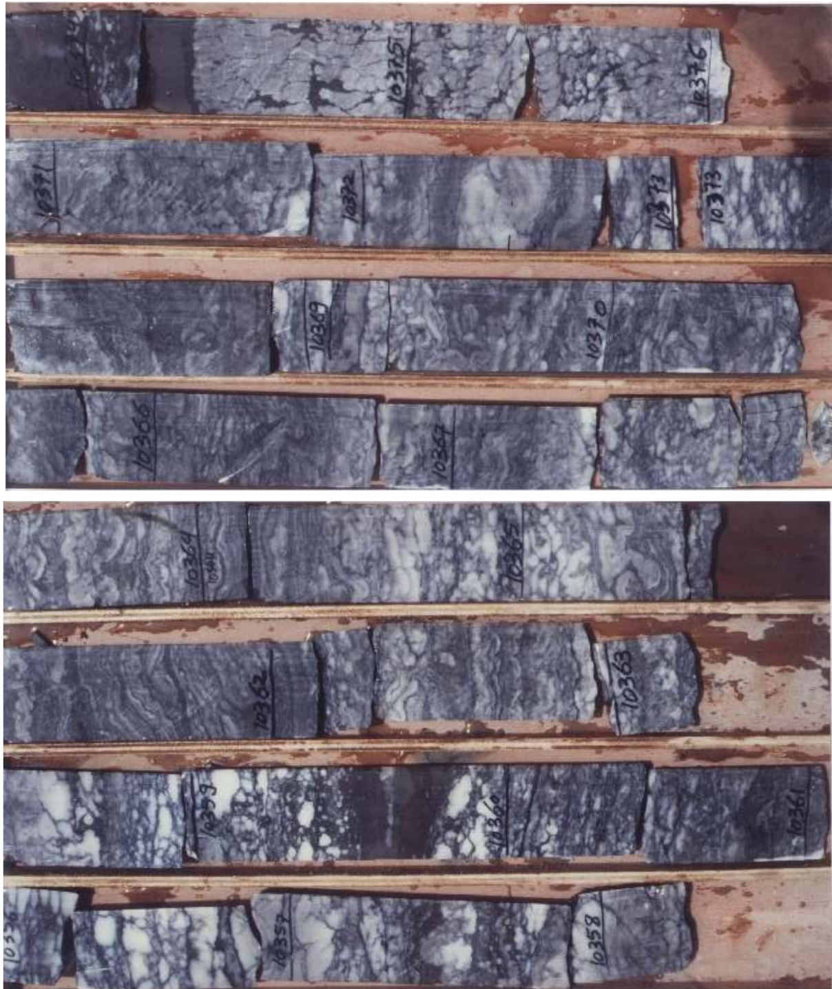
Figure 11: Cores from part of the Upper Anhydrite, Arab Formation, showing 24 feet of nodular, laminated and enterolithically folded anhydrite. Note the significant thickness of vertically continuous anhydrite. Note also the well developed subvertical anhydrite nodules at approximately 10,375 feet.
