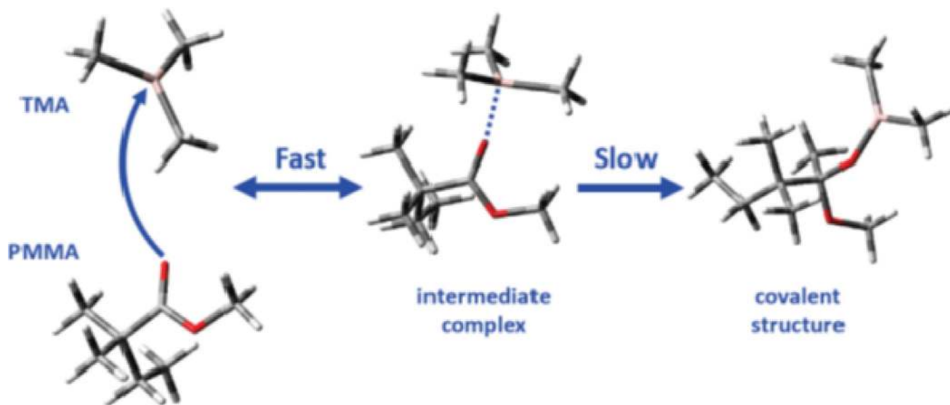
Figure 4. Proposed mechanism for TMA reaction in PMMA. PMMA and TMA interact rapidly and reversibly to form a weakly-bound complex, but the subsequent reaction to form the covalent structure is slow.
