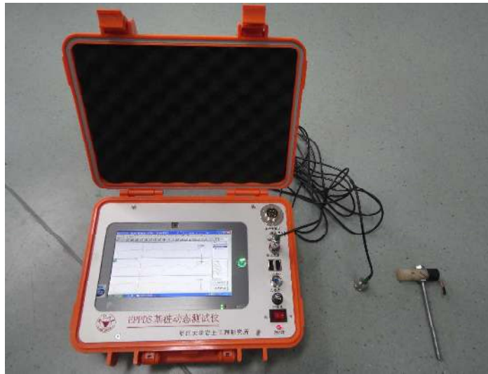
(b) EPPDS Dynamic Testing System of Pile
