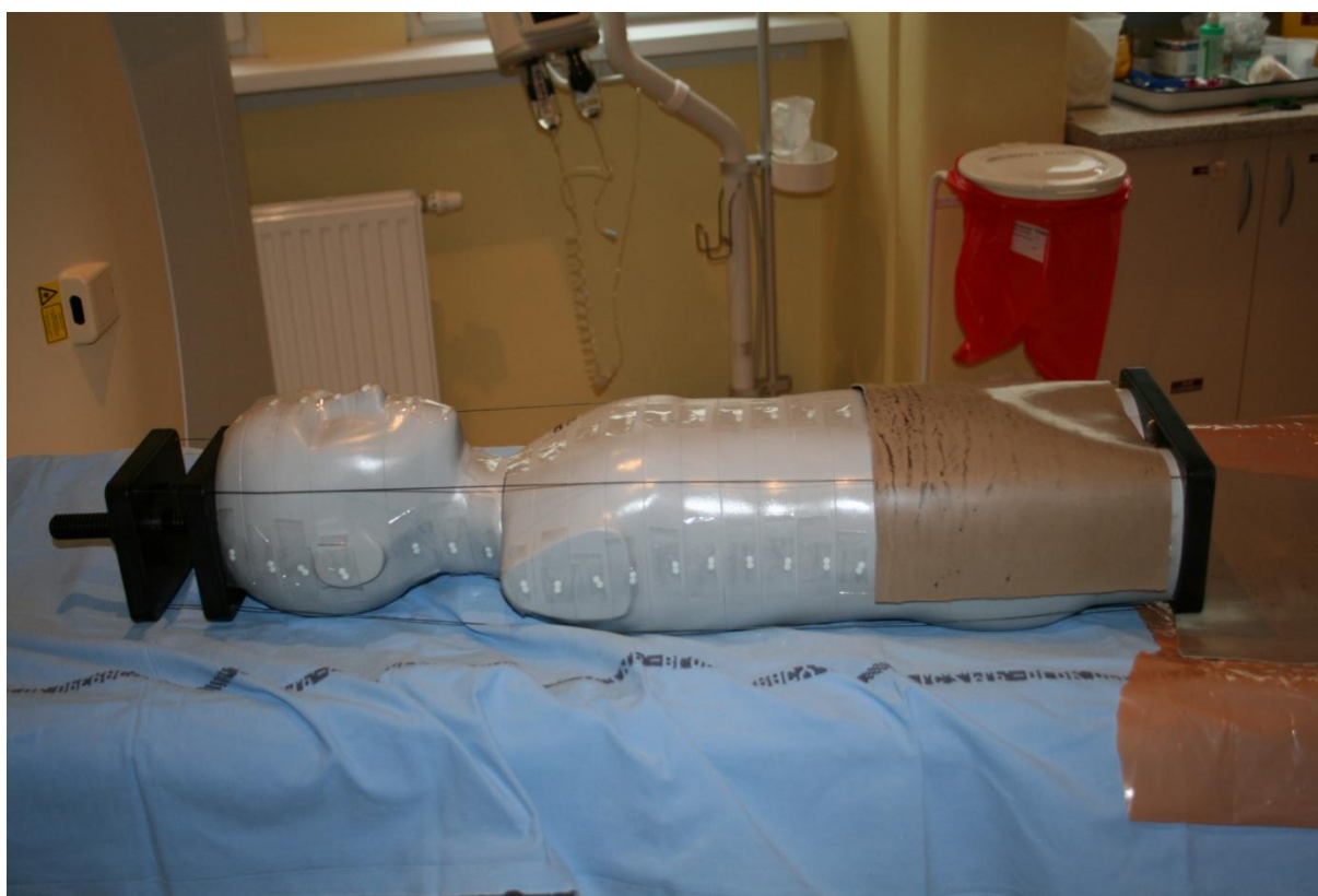
Fig. 3 A phantom imitating a 5-year-old child with the shield placed on its surface.
