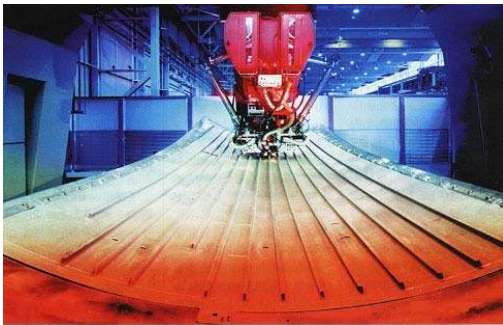
Fig. 1 Laser beam welding aircraft fuselage Fig. 2 Fuselage joined with friction stir welding
