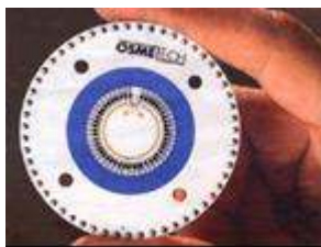
Figure 16.5 - The analyzer instrument consists of conductive polymer sensor elements, made using wafer scale technology [36]
