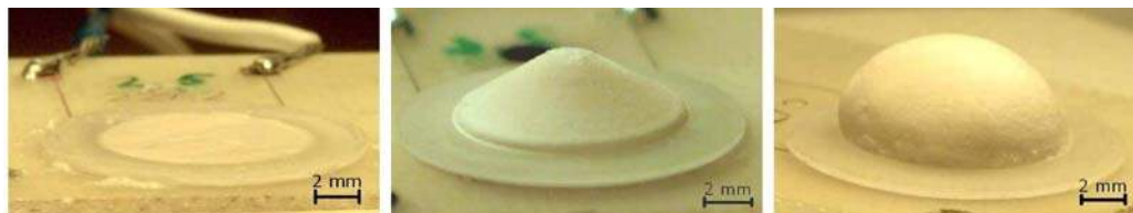
Figure 11.9: Photographs showing the paste a) unexpanded (state before actuation), b) expanded (state after actuation; liquid container removed for visualization) and c) expansion without constraining liquid container results in a volume expansion of seven times the original volume [5].
