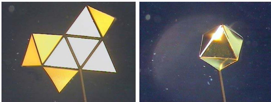
Figure 13.7. A self assembling octahedron controlled by several hinge actuators
