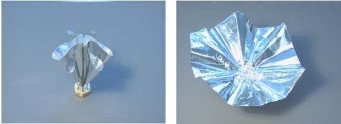
Figure10. 2: SMA actuator activated with solar energy. When the sun illuminates the structure, the SMA ribs bend and open the highly reflective surface (4cm diameter) to the sun. [50].
