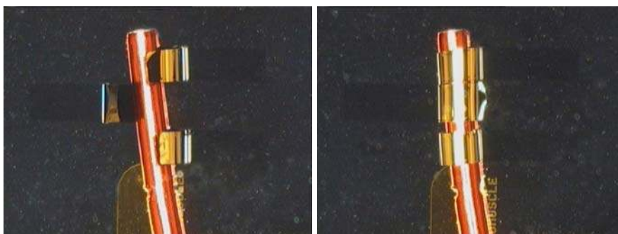
Figure 13.5 - Three bilayer actuators (500 \mu\text{m} wide) grabbing a 0.5 mm wire
