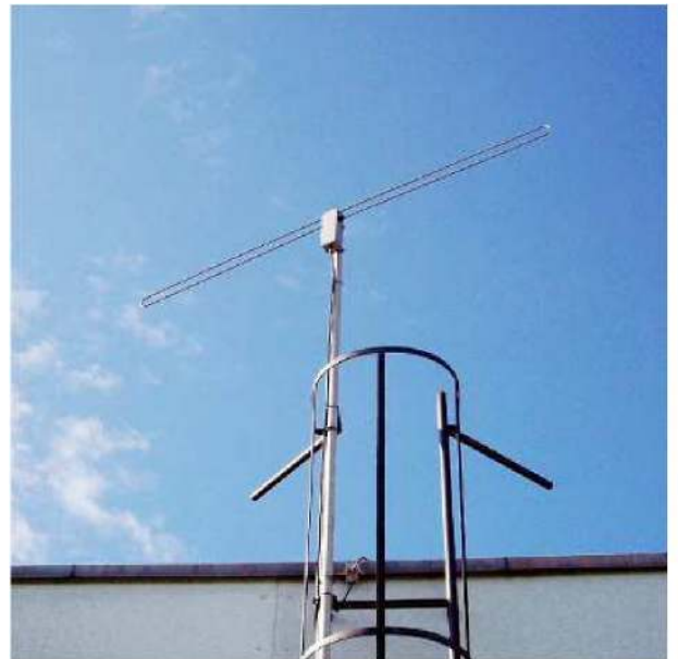
Figure 8: The dipole antenna used as beacon to monitor the timing of LOPES.
