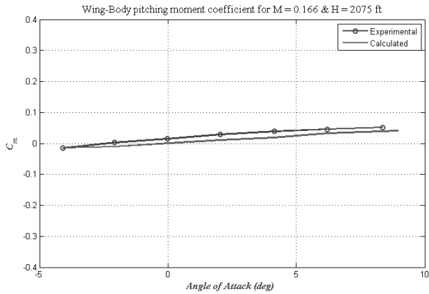
Figure 7. C_m versus \alpha (experimental and calculated), WB configuration.
