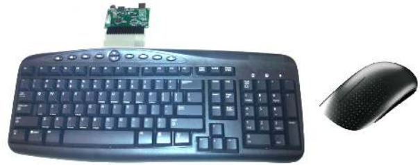
Fig. 8: A regular mouse and keyboard can be used to assess stress through behavior. This hardware can also be modified to provide additional features. The image depicts a pressure-sensitive keyboard and a capacitive mouse [89].
