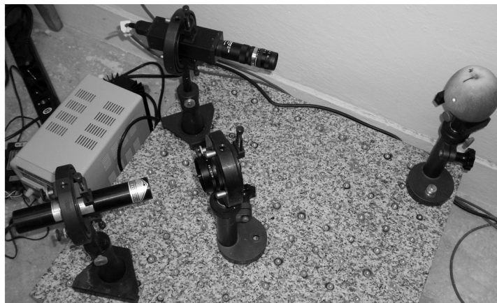
Fig. 3. Experimental setup for studying of apple specimen biospeckle temporal properties.
