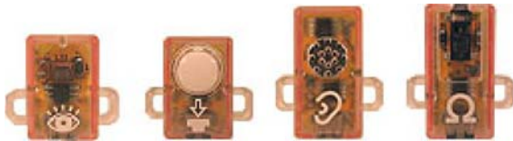
Fig. 5 PicoCricket sensors: light sensor, touch sensor, sound sensor, resistance sensor
