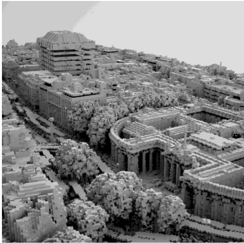
Fig. 16. Octree applied to LiDAR data set.
