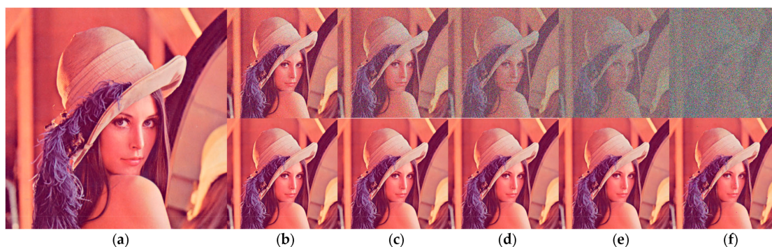
Figure 6. Qualitative evaluation of the NFMO performances applied to the Lena 512 \times 512 color image. (a) Original Lena image. Top (b–f) Noised Lena images with noise density 10%, 30%, 50%, 70%, and 90%. Down (b–f) Filtered Lena Images by NFMO.
