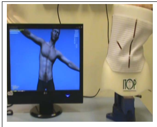
Figure 4. Bend sensors are applied on garments to measure trunk postures. A 3D avatar furnishes a visual feedback.
