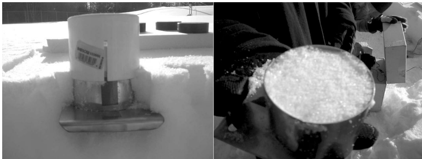
Fig. 2. The IRIS sampler before extraction of the snow sample within the snow cover (left) and after the sample extraction with the cut surface (right).
