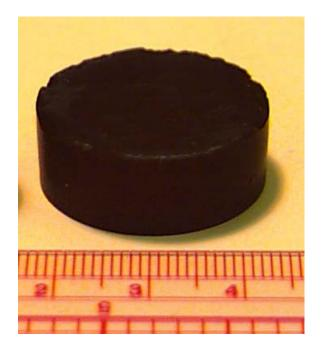
**Figure 1.** Photo of chromia aerogel monolith ( $\rho = 280 \text{ mg/ml}$ ). The scale of the ruler in the photo is in cm.
