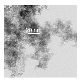
Figure 2. A high-resolution transmission electron micrograph of a chromia aerogel.
