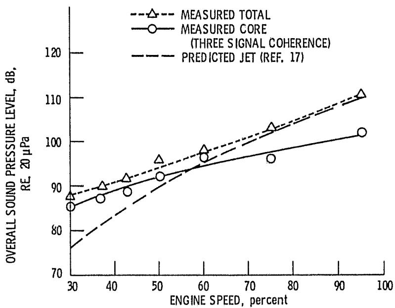
Figure 11. - Variation of measured total and core and predicted jet noise overall sound pressure levels with engine speed at  $120^{\circ}$  from engine inlet, (frequency range 50-1000 Hz).
