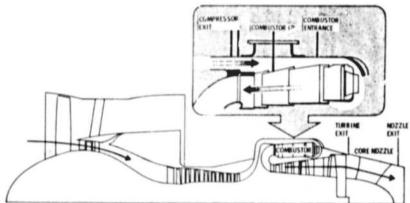
Figure 4. - Schematic showing core probe locations.
