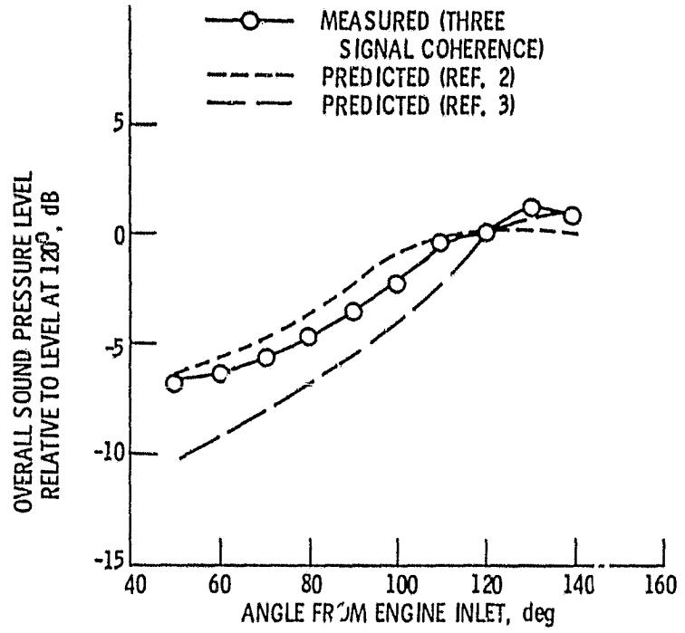
Figure 17. - Comparison of measured and predicted overall sound pressure level directivities, 30% engine speed.
