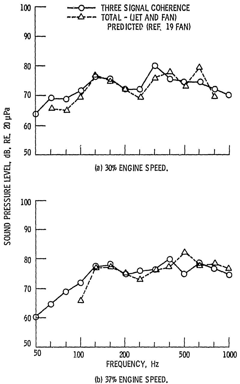
Figure 14. - Comparison of core noise measured using three signal coherence technique with core noise estimated by subtracting jet and fan noise from the measured total noise using reference 19 fan noise prediction,  $120^{\circ}$  from engine inlet.
