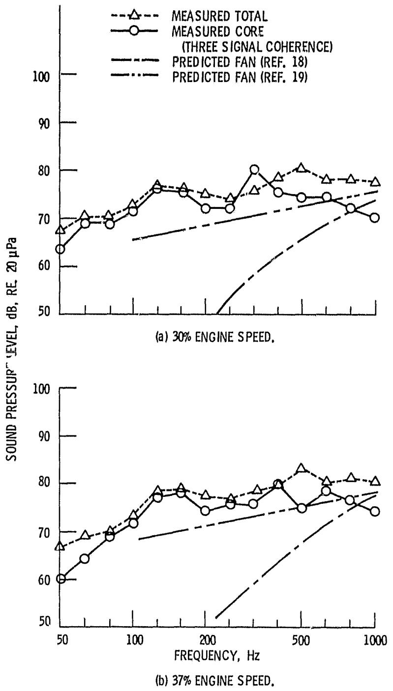
Figure 13. - Comparison of fan noise predictions using method of references 18 and 19 with measured core and total noise at  $120^{\circ}$  from engine inlet.
