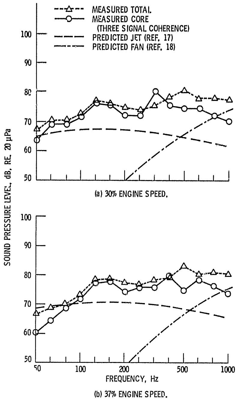
Figure 10. - Comparison of core, jet, and fan noise levels to total noise at  $120^{\circ}$  from the engine inlet.
