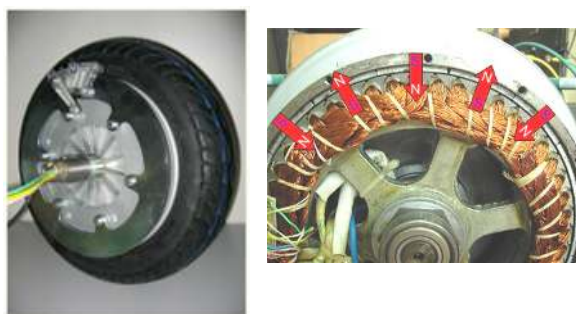
Inner view of the wheel motor with pole direction
