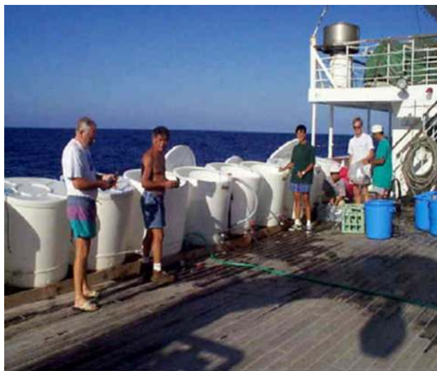
Fig. 4 Large volume plastic containers (400 L) on the shipboard for scavenging of ^{90}\text{Sr} , ^{137}\text{Cs} , Pu isotopes and ^{241}\text{Am} from seawater samples (IAEA'1997 cruise [22])
