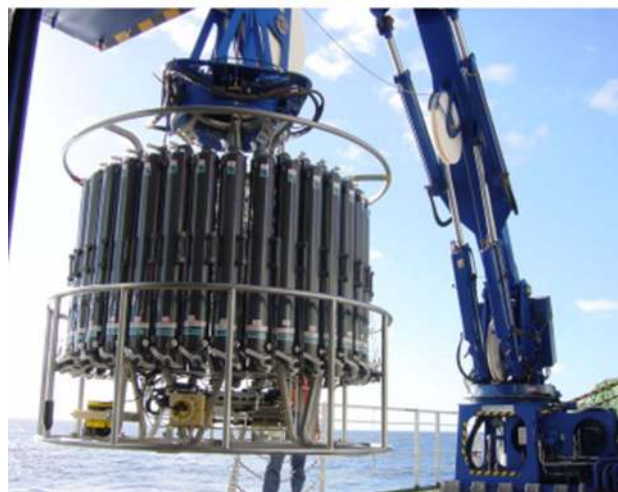
Fig. 3 Large-volume (200 L) water samplers (top) compared with the Rosette multisampling system (24 bottles with 20 L volumes) (bottom) operating during deep-water sampling in the Pacific Ocean (IAEA'1997 cruise [22])
