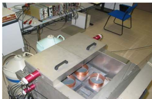
Fig. 11 Lead shield with four Ge detectors operating in a shallow underground laboratory in IAEA Monaco with antic cosmic shielding made of plastic scintillators [39]
