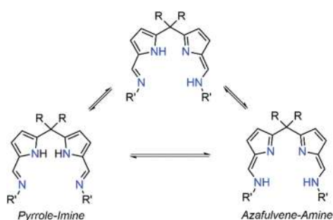
Scheme 1 Possible pyrrole-imine to azafulvene-amine tautomerization (single and double).
