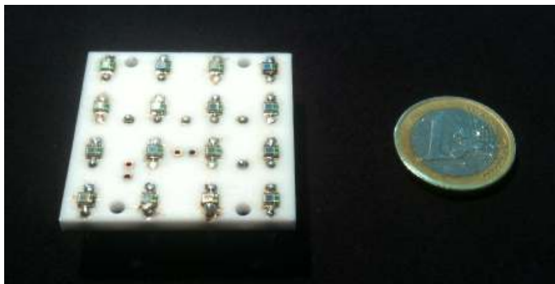
Figure 11. Dice Board, used in NEXT-DEMO, containing 16 (4×4) MPPCs.
