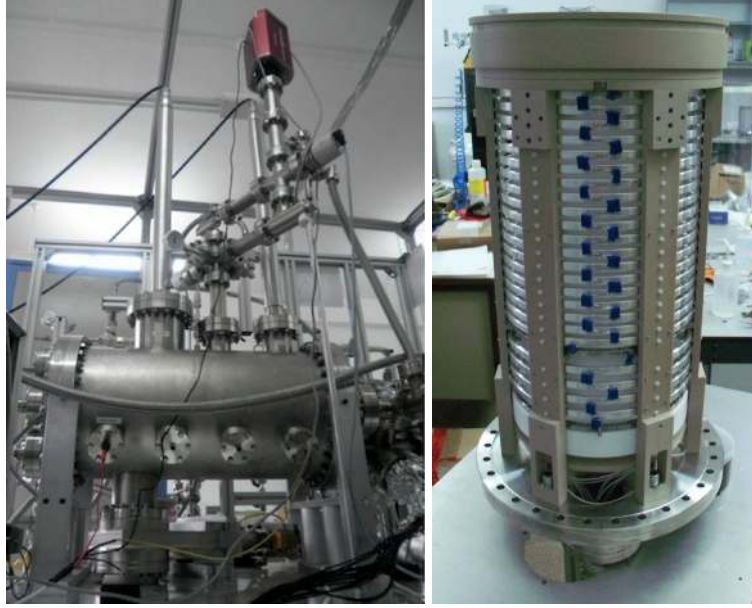
Figure 4. The NEXT-DEMO prototype, operating at IFIC. Left: the pressure vessel. Right: the time projection chamber.
