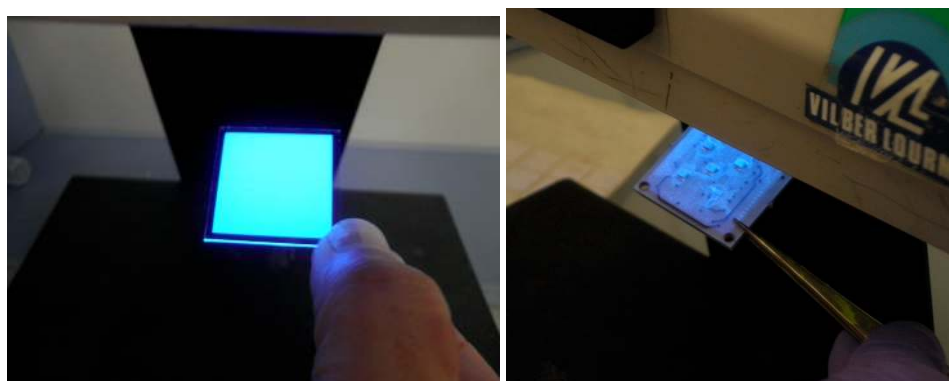
Figure 12. Illumination with 240 nm UV light of a glass-slice (left) and a 5-SiPM board (right) both coated with TPB.
