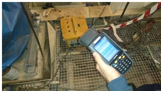
FIGURE 14: Tag reading in an area of very high density of metallic objects.
