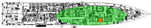
FIGURE 15: Blueprint of the OPV showing the active UHF RFID coverage (horizontal projection).
