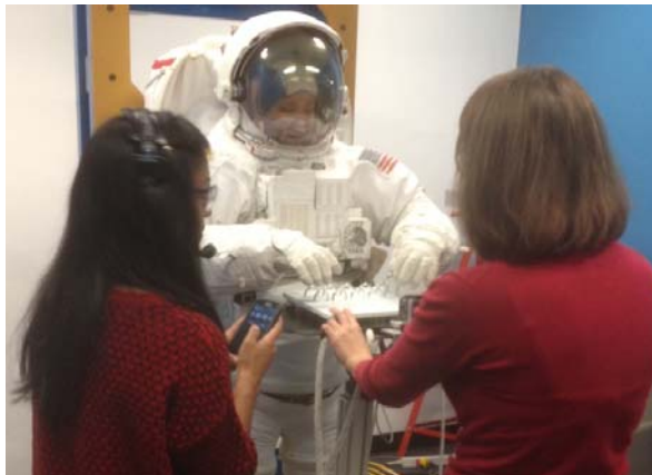
Figure 9. Evaluating protocols for assessments of glove mobility. Test subject in pressurized suit performing “Pin” task.
