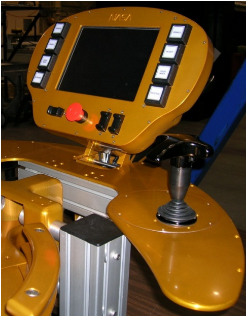
Figure 15. Console – crew accommodation system.
