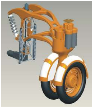
Figure 5. Wheel module with suspension.
