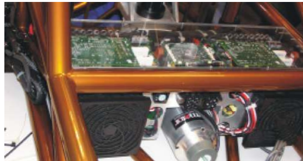
Figure 11. Powertrain control module – installed with plexiglass cover.
