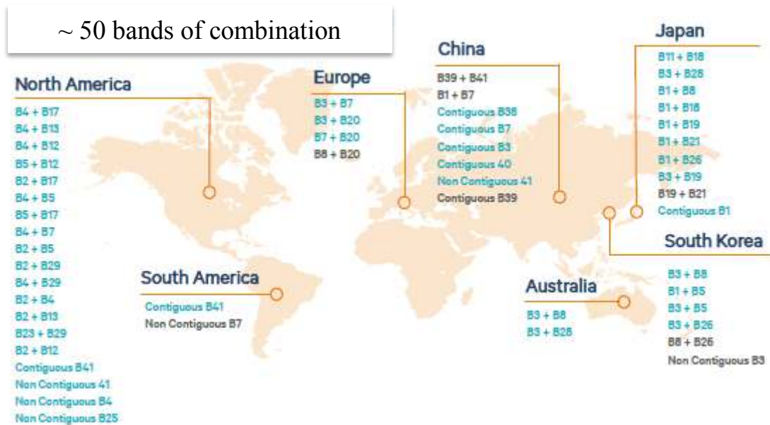
Fig. 2.14 Samples of the supported LTE CA channels from a commercial design.
