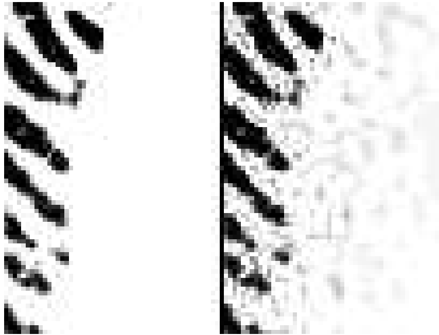
Figure 72: Artifacts at the boundary of a fingerprint resulting from WSQ compression (factor 8) after setting gamma value to 0.1.
