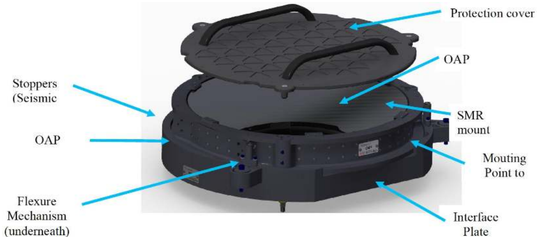
Figure 7: OAP mirror cell with interface plate
