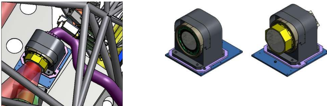
Figure 3 Tip Tilt Stage can carry DM11 in case of DM0 failure. The left figure shows the TTS in NFIRAOS in the fall-back position with the TTS moved back and DM11 extending in front of the stage. The middle image shows the baseline configuration with DM0 mounted on the TTS, and the right shows the repair position.
