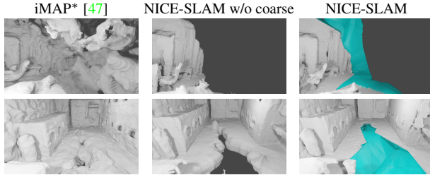
Figure 7. Geometry Forecast and Hole Filling. The white colored area is the region with observations, and cyan indicates the unobserved but predicted region. Thanks to the use of coarse-level scene prior, our method has better prediction capability compared to iMAP*. This in turn also improves our tracking performance.
