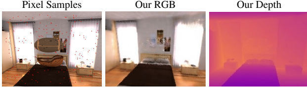
Figure 6. Robustness to Dynamic Objects. We show the sampled pixels overlaid on an image with a dynamic object in the center (left), our rendered RGB (middle) and our rendered depth (right) to illustrate the ability of handling dynamic environments. The masked pixel samples during tracking are colored in black, while the used ones are shown in red.
