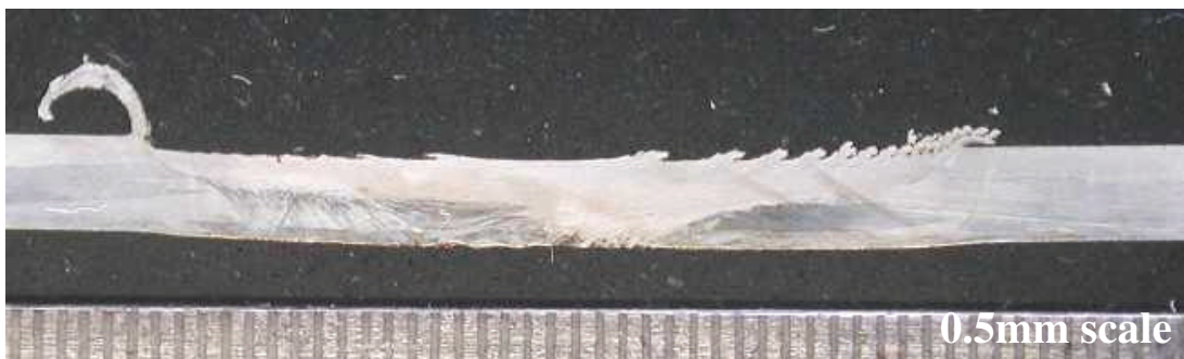
Figure 20. Friction stir welding of ODS MA956 alloy sheet.
