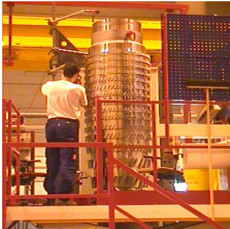
Figure 14. ALSTOM Power GTX100 EB-welded compressor rotor assembly.
