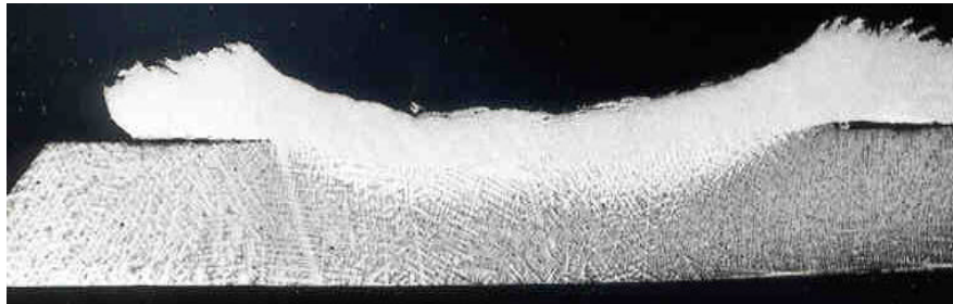
Figure 19. IN939 Hopkinson 1-shot technique friction welded section [14].
