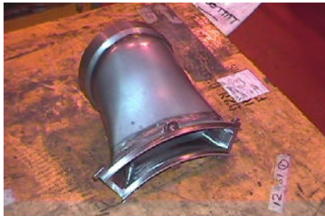
Figure 7. ALSTOM Power UK Haynes 230 transition duct.
