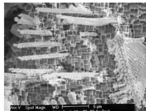
Fig. 3 SEM micrographs of a) blocky, b) script, and c) nodular MC carbides contained within the interdendritic regions of carbon-containing Ni-based superalloys.
