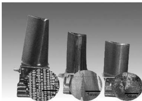
Fig. 8 Grain structures of single-crystal, directionally solidified, conventionally cast turbine blades.
