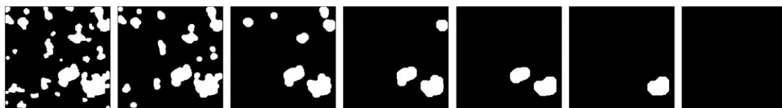
Fig. 3 Particle size distribution obtained by consecutive opening (with octagon as structuring element).
