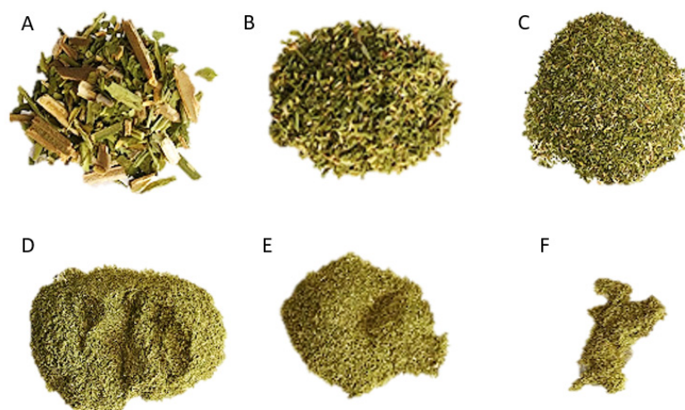
Figure 4. N. tabacum var. Virginia leaf waste powder. Sieved fractions from ground leaf waste. (A) 840 \mu\text{m} . (B) 500 \mu\text{m} . (C) 149 \mu\text{m} . (D) 105 \mu\text{m} . (E) 74 \mu\text{m} . (F) <74 \mu\text{m} .
