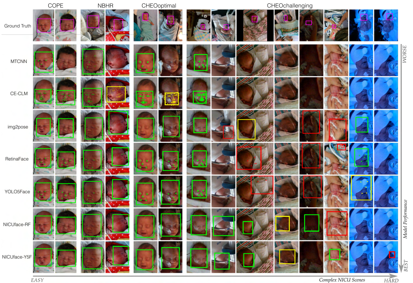
FIGURE 4. Face Detection Results from all neonatal datasets, pretrained models, and NICUface models. Increasing level of scene complexity is demonstrated from left to right. Increasing performance of each model is presented from top to bottom. Predictions are labelled as correct ( IOU \geq 50 , Green), partial ( IOU \geq 30 , Yellow), or incorrect ( IOU < 30 , Red).
