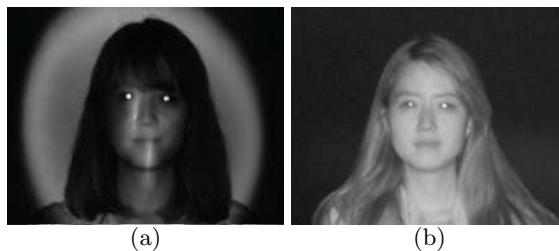
Fig. 2. Nighttime NIR images at 60m acquired using (a) the NIR illuminator used in [19] and (b) an improved illuminator used in this paper. Notice the noisy light pattern around the head in (a) generated by the NIR illuminator in [19].
