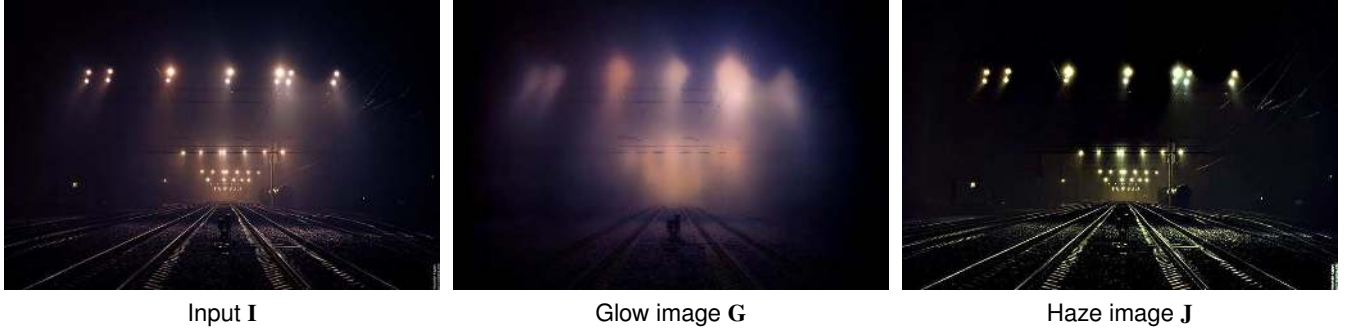
Figure 6. Glow decomposition results. (Left column) shows the input images. (Middle column) shows the estimated glow images. (Right column) shows the estimated haze images. As one can notice, the presence of glow in the haze images is much reduced.
