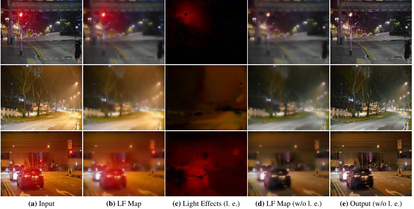
Figure 4. Examples showing the suppression of light effects from our method. (a) Input image. (b) Sample LF feature map obtained from the image. (c) Generated map showing glow/glare/floodlight light effects. (d) Sample LF feature map after subtracting the light effects map. (e) Output image with suppressed light effects. Note that, the output images shown are not with increased dynamic range.
