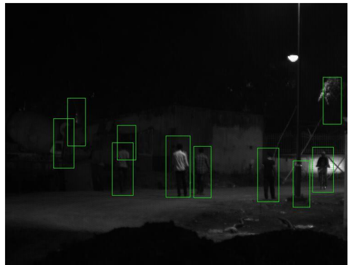
Fig.2 Output of the Haar cascade Detection stage which contains several False alarm.
