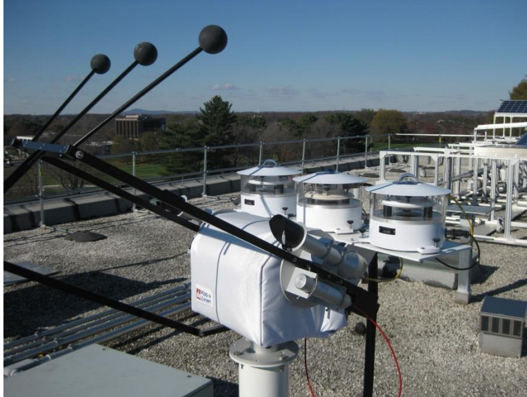
Figure 3-3 The pyrheliometers mounted on the solar tracker above the sun sensor and below the horizontal diffuse-measuring pyranometers (left and right) and IR measuring pyrgeometer (center). The black balls shade the three horizontal instruments.
