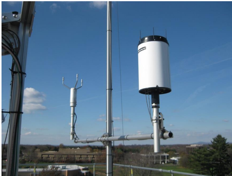
Figure 3-6 The lower ultrasonic wind sensor (left) and heated tipping bucket rain gauge (right) on the lower instrument mast crossarm
