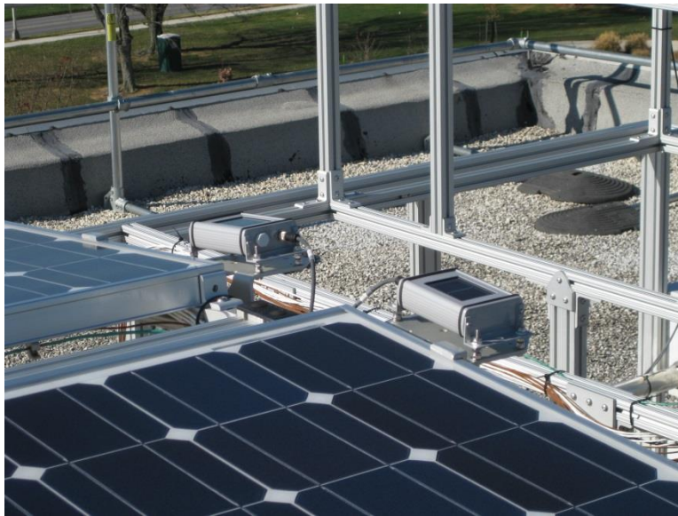
Figure 3-2 Flat-plate silicon irradiance sensors measuring the POA irradiances on their respective reference modules
