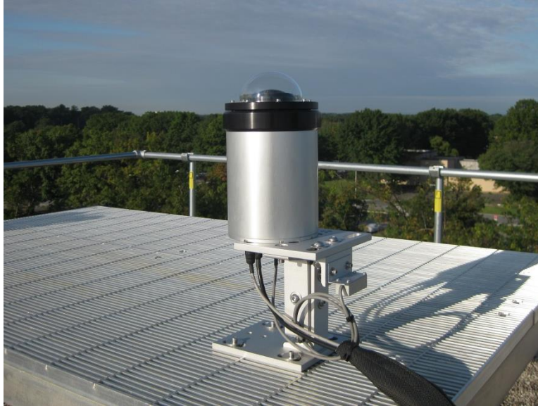
Figure 4-6 The all sky camera with the ambient temperature and humidity sensor installed on a custom mount on the west table
