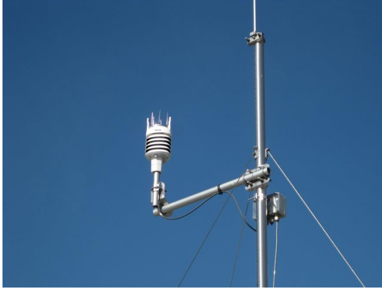
Figure 3-5 The weather transmitter near the top of the instrument mast
