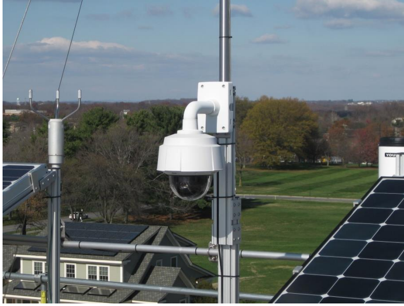
Figure 4-5 The PTZ camera that records images of the instruments and NZERTF PV array
