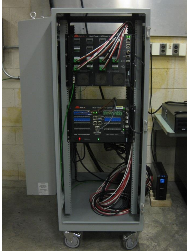
Figure 4-4 The I-V curve tracer with maximum power tracker and load
