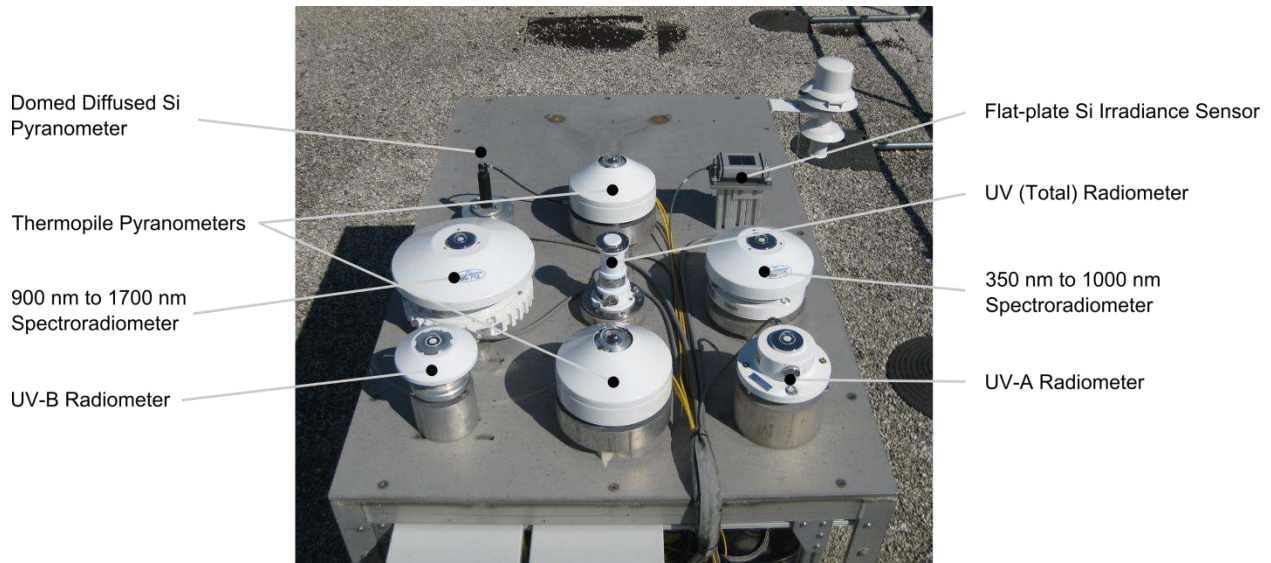
Figure 3-1 The east table, looking north, with the GHI measuring pyranometers and silicon irradiance sensor mounted on it. Also shown are the spectroradiometers, UV radiometers, and the ambient temperature sensor (upper right).
