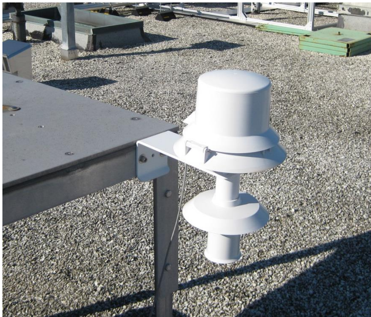
Figure 3-4 The temperature sensing probe in the aspirated radiation shield used to measure the outdoor ambient air temperature
