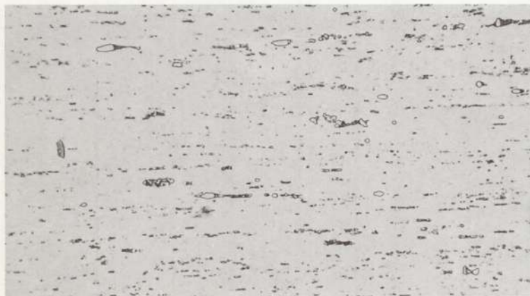
(C) COMPOSITION C NITINOL WIRE, 100-MIL DIAMETER, 10% REDUC- TION
