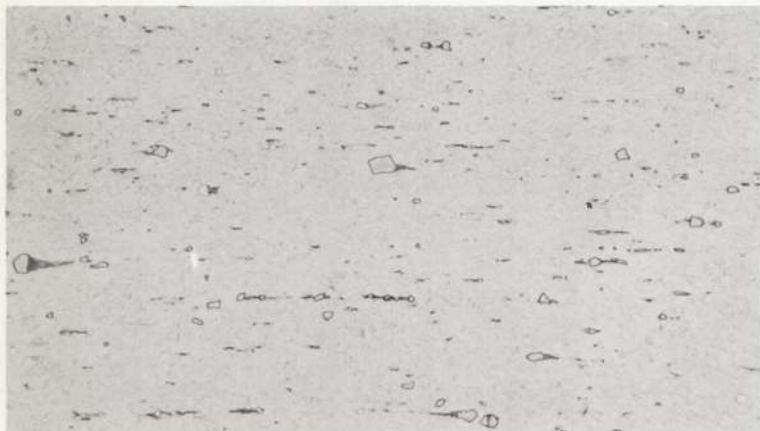
(B) COMPOSITION B NITINOL WIRE, 20-MIL DIAMETER, 20% REDUC- TION
