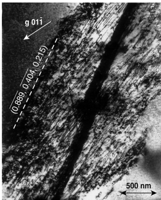
Fig. 2 Large array of dislocation loops in the cubic austenite phase of the \text{Ni}_{50.5}\text{Ti}_{49.5} specimens after one thermal cycle that was imaged near [111]_A with g\ 01\bar{1} . Under these imaging conditions, the dislocation line directions, \mathbf{u} , are parallel to [020]_A and are perpendicular to the foil surface; hence the dislocations have a screw character. The strong-contrast dislocation band through the array is composed of mixed orientations and is parallel to (0.889, 0.404, 0.215) , according to Ref 5
