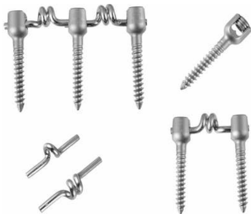
FIG. 1. Photographs showing the components of the BioFlex dynamic stabilization system, which is composed of titanium screws and Nitinol rods. The rods are of two types, one with a single turn forming the coil and one with two turns in the coil. In the upper right corner the photograph shows the BioFlex screw head design. Its two grooves enable insertion of two rods per segment in cases in which more than one segment is stabilized. (Reprinted with permission from Bio-Spine Corp.)
