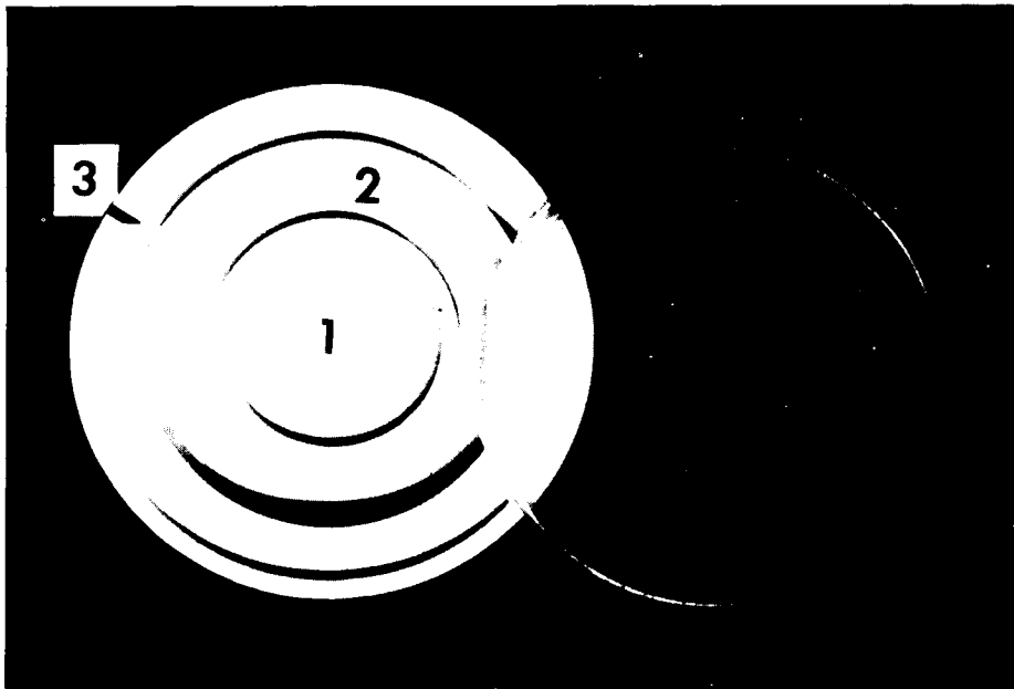
FIG. 1—The Obrink modification of the Conway microdiffusion dish, showing the central boric acid chamber (No. 1), the peripheral sample chamber (No. 2), and the annular moat (No. 3). The clear polypropylene cover, when seated in the moat, seals off the acid and sample chambers.
