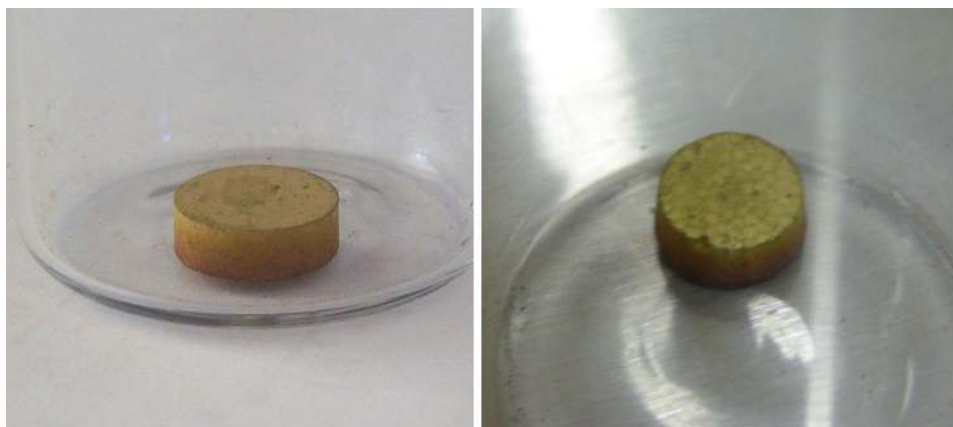
Fig. 10 Comparison between two ZrN pellets sintered at 2000 °C. There is a distinct difference observable by ocular inspection between the pellets based on if the microspheres pressed were destroyed or retained their individual shape during compaction [50]
