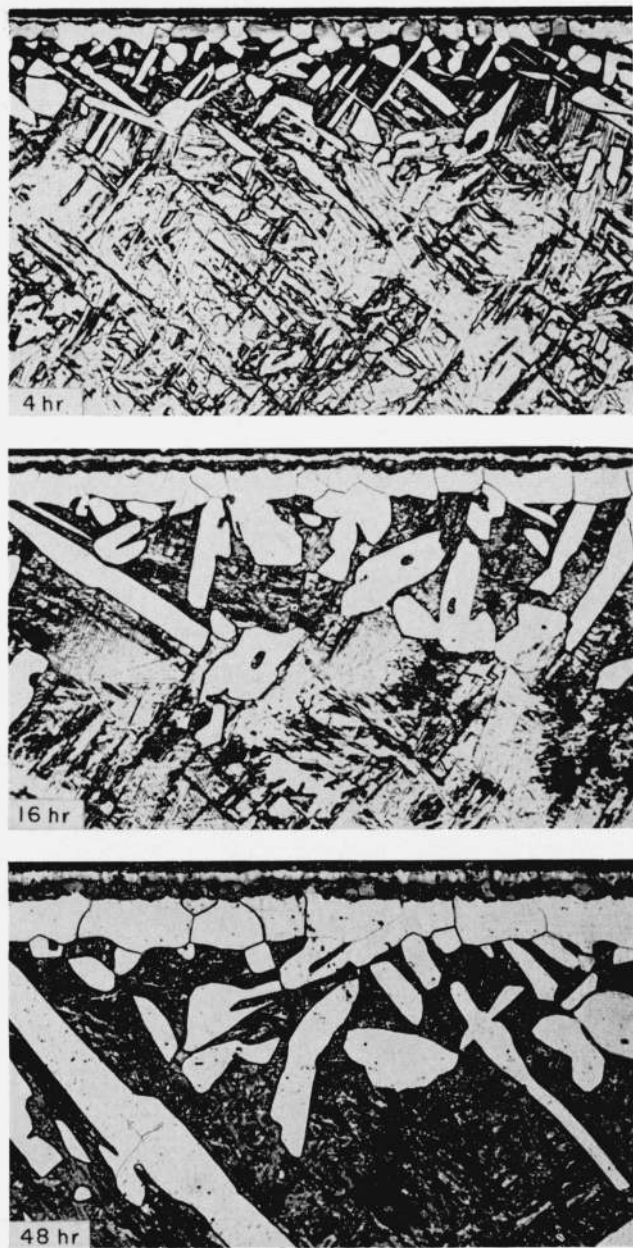
FIGURE 3. 6Al-4V titanium alloy nitrided in purified nitrogen at 1,800° F for the lengths of time indicated.
