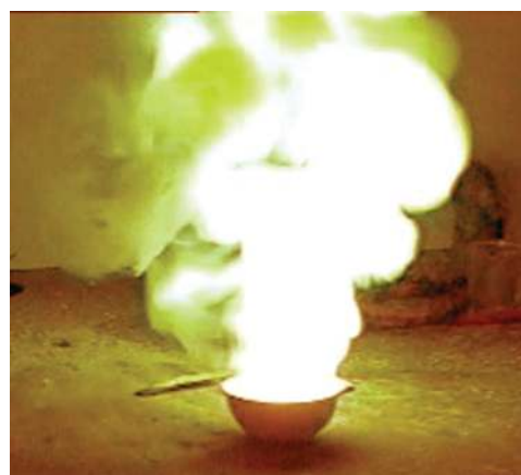
Fig. 1. \text{Zn} + \text{S} \rightarrow \text{ZnS} . Photo by Kevin A. Boudreaux. [1] Reproduced with permission.
