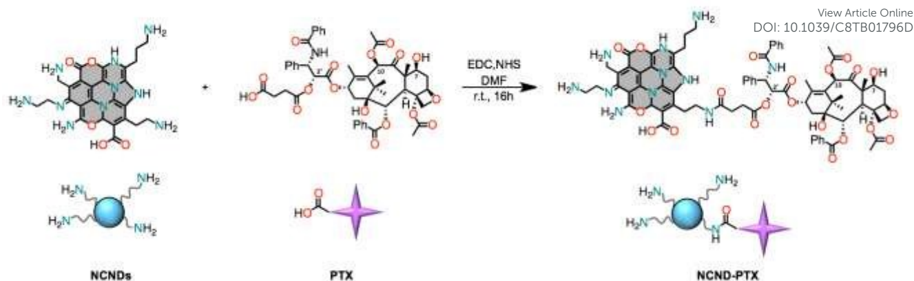
Figure 1. Synthetic scheme for the covalently linked nitrogen-doped CNDs (a representative structural unit is depicted)-paclitaxel (NCND-PTX) used in this study.
