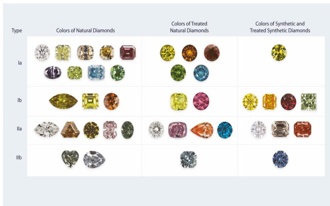
Figure 4. Diamonds exhibit many different colours depending on their impurity levels. Reprinted and adapted with permission from Ref.10. Copyright © 2009 Gemological Institute of America.
